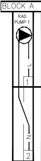
The only high voltage connection to be made apart from the power supply is connecting the radiator pump on block A. Use one of the cable fittings at the top for cable penetration. The earth wire is connected directly to the earth block.
