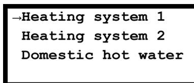
**House heating (1):** This is where you adjust the settings for controlling the heating system, including manually adjusting the heating curve.
