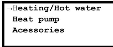
**Heating / Hot water:** Here you see the current values for the tank temperatures, the temperature of the water in the radiators / underfloor heating, room temperature, etc.
