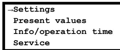
**Settings:** This is where you can adjust the settings for the heating curve, among other things, and set the room temperature and the domestic hot water temperature, etc.
