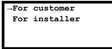
**For customer:** This is where you can adjust the settings for the heating curve, among other things, and set the room temperature and the domestic hot water temperature, etc.
