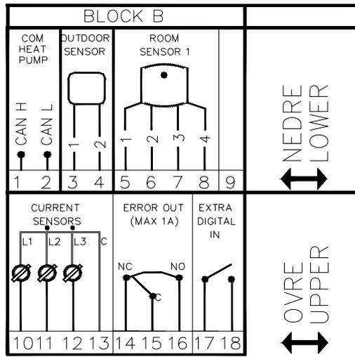
Block B contains all of the low-voltage connections that are included as standard with the Exotic Compact. Some of the connections do not need to be connected for the product to work.
