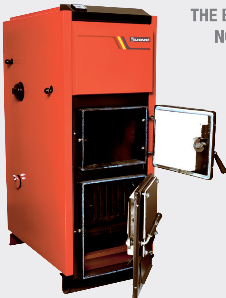
Exonom P20 UB. Doors with mounting plates for pellet burner, ceramic insulation on the inside, grate (removed for pellet and oil burning), wood burning grate and ash box.
